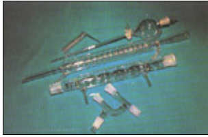
Liebig condenser, Dimroth condenser, Allihn condenser
